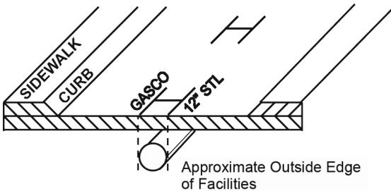
These examples indicate an operator's 12 in. facility. When a facility can be located or toned separately from other facilities of the same type, it is marked as a single facility.<sup>41/</sup>
